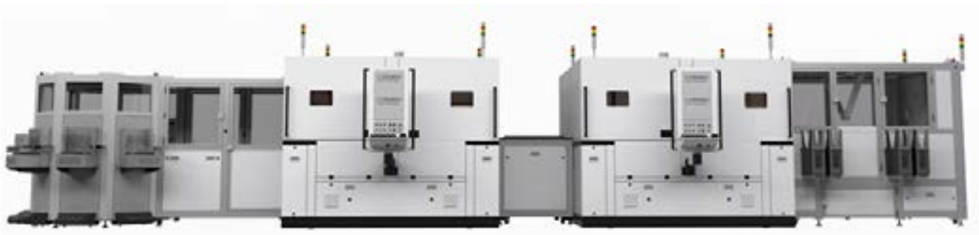
Figure 2: Fully automated process solution by CLT to singulate eyepieces from a wafer to a part.
