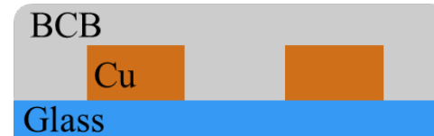
Cross section view of interdigitated test structure (IDT) with and without silicon nitride barrier layer
