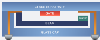
Core Switch Simplest, smallest building block can be integrated into many power or RF applications.
