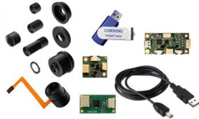
Figure 8 : D-u-25H0-075-03 development kit provided by Corning® Varioptic®
