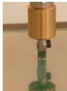
Figure 2. A photo of a score wheel in the process of creating a median crack
