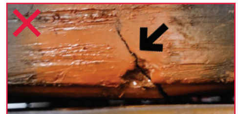
Large (greater than 1/16 inch) cracks in side or edge of flange
