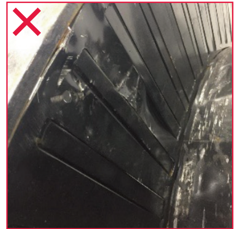
Material with dents or damage on the flange.
