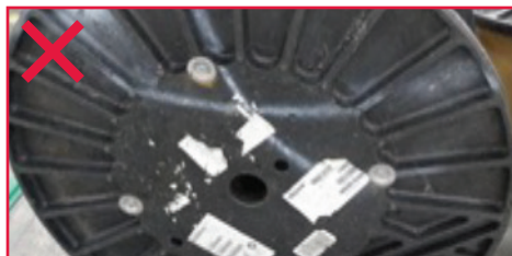
Paint and labels on the outside of the flange
