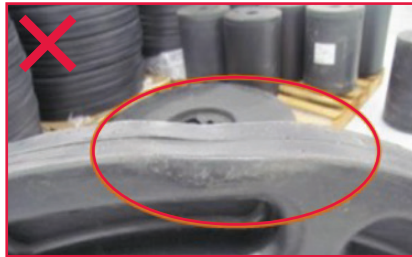
Flanges with dents or warping
