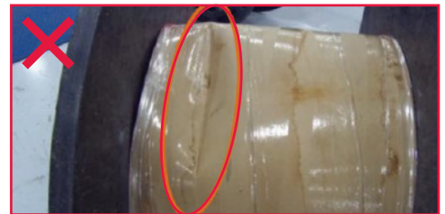
Drum with greater than 6-inch dent
