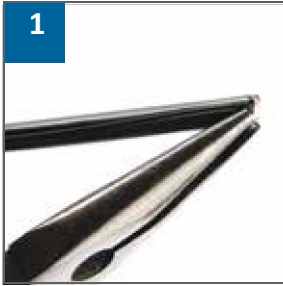
Figure 12. Advanced Stripping Process Starts With Commonly Used Hand Tools to Initiate Jacket Peel
