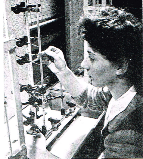
Amelia Maio inserts a specified amount of liquid into pipette in CGW apparatus department to determine accurately the graduations to be engraved into the glass. The pipette, in turn, is used to measure Penicillin solutions in the assay laboratories
