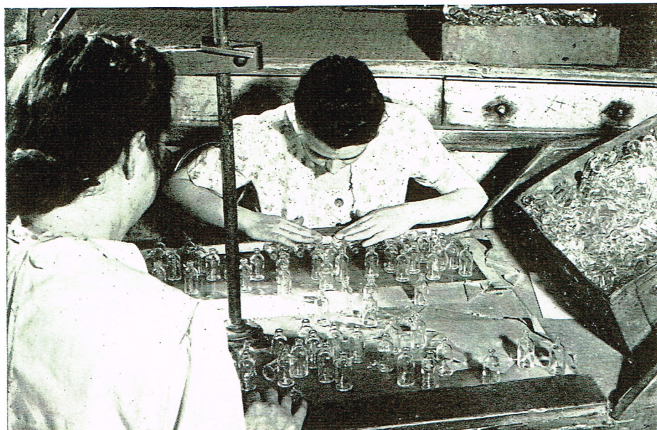
Final inspection and packing of Penicillin dispensing bottles is done in Pyrex finishing by Elizabeth Teets and Martha Bohart
